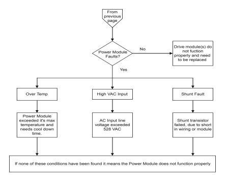
Figure 60: Power Up Sequence Flow Chart - Part 2
