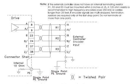
Figure 47: Command Connector (J5) Encoder Output Wiring
