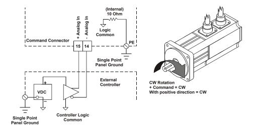
Figure 45: Analog Command, Differential Wiring Diagram
