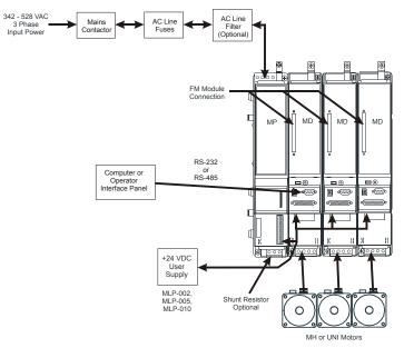
Figure 1: Module Drive System Overview
