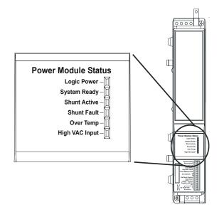
Figure 34: Power Module Status Indicator location
