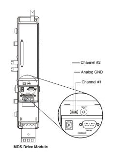
Figure 65: Diagnostic Analog Output Test Points
