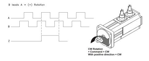
Figure 48: Direction Convention Diagram
