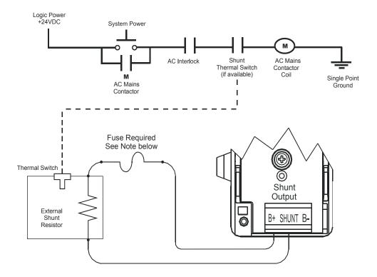
Figure 23: Power Module Shunt Wiring
