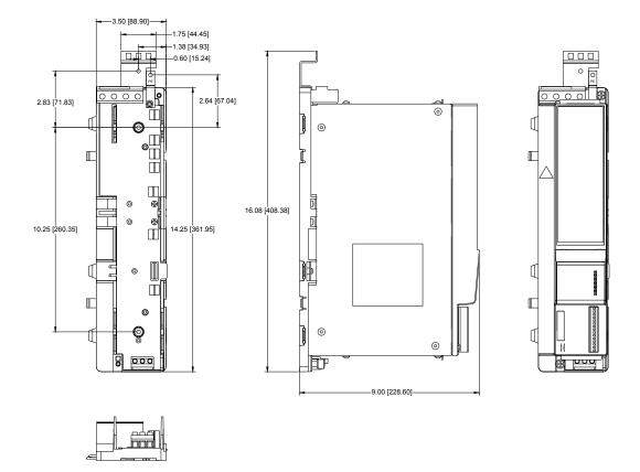
Figure 73: MP-5000 Dimensional Drawing
