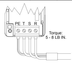
Figure 26: Drive Module Motor Power Wiring Diagram
