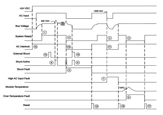
Figure 38: Power Module Logic Timing Diagram
