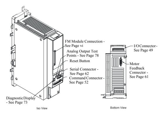
Figure 39: Drive Module Operations and Features
