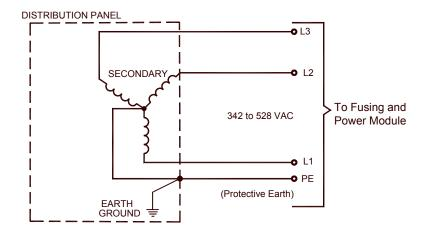
Figure 16: Earth Grounded WYE Distribution Transformer
