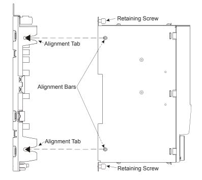
Figure 27: Power Module Assembly Diagram
