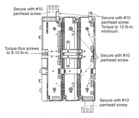
Figure 13: Securing the Drive Module backplane to the Power Module backplane.
