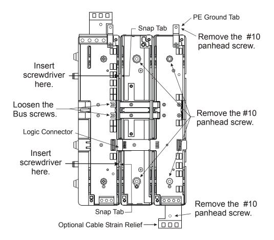
Figure 64: Drive Module Backplane Disassembly Diagram
