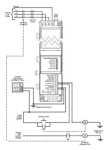
Figure 37: AC Interlock with 120/240VAC Mains Contactor
