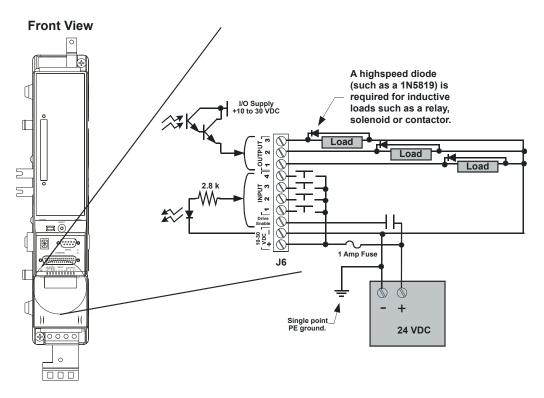
Figure 40: MDS Drive Module Input/Output Wiring Diagram
