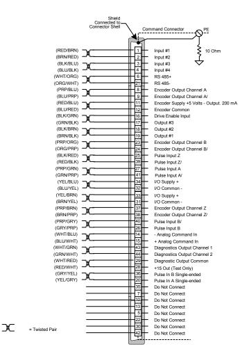
Figure 44: Command Connector (J5) Pinout and CMDO-XXX Wire Colors
