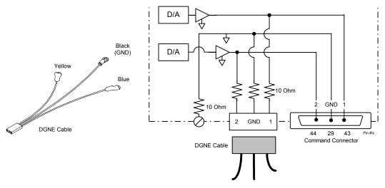
Figure 66: Diagnostic Cable (DGNE) Diagram
