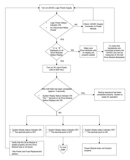
Figure 59: Power Up Sequence Flow Chart - Part 1
