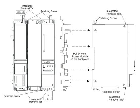
Figure 62: Power and Drive Module Removal Diagram
