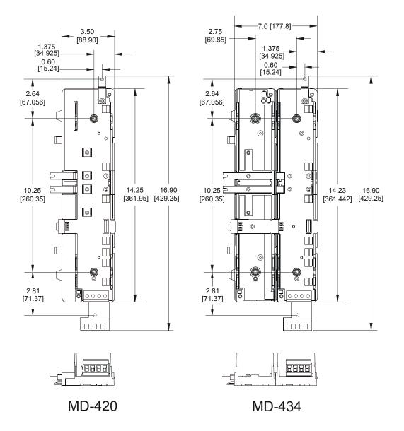
Figure 9: Drive Module Backplane Dimensions
