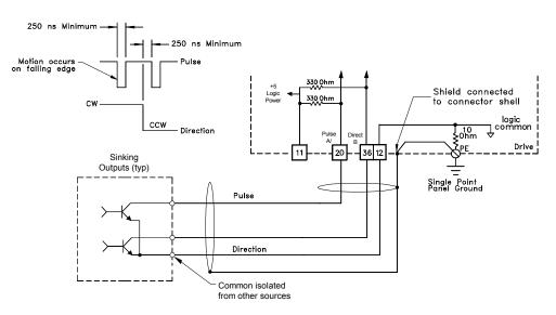
*Figure 52:* Pulse Mode, Single Ended Output to Single Ended Input (non-twisted pair cable)
