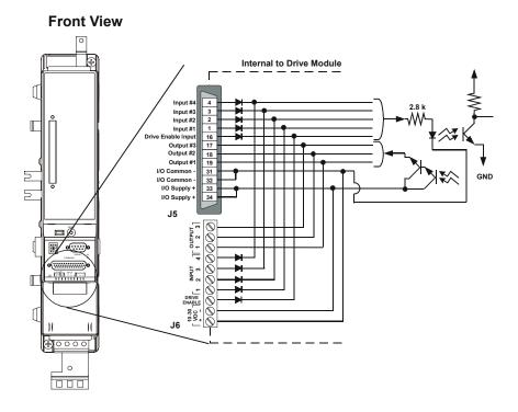
*Figure 41: MDS Drive Module I/O Connector to Command Connector Internal Connections*
