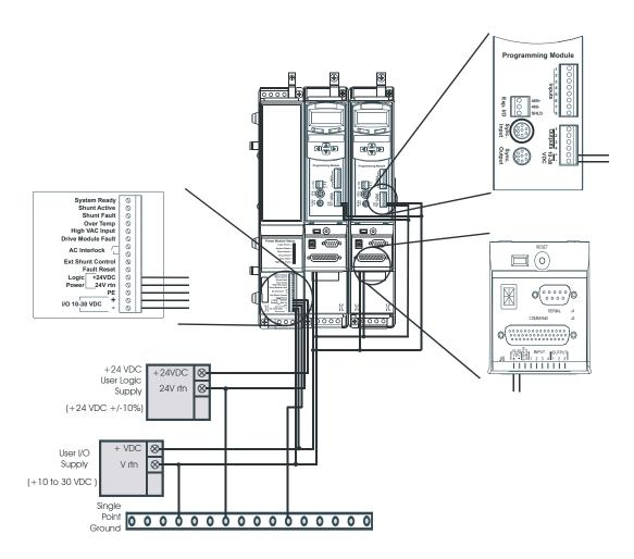
In Figures 31 and 32 the MDS Logic and I/O power are separated for applications that have Digital I/O power (+10 to 30VDC) that is out of the Logic Power Range (+24VDC +/-10 %).
