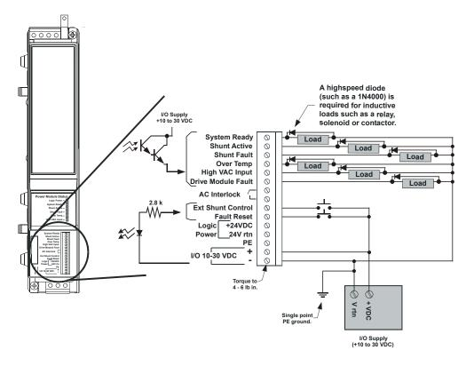
Figure 35: Power Module I/O Wiring Diagram
