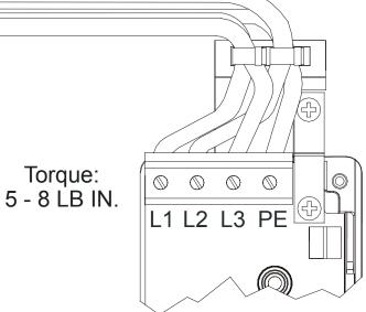
Figure 21: Power Module AC Power Wiring Diagram
