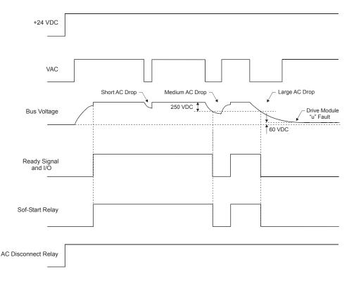
*Figure 61: AC Glitch Handling Diagram*
