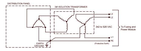
*Figure 18:* Three Phase Delta (with mid-phase GND) Distribution to a Three-Phase WYE/WYE Isolation Transformer
