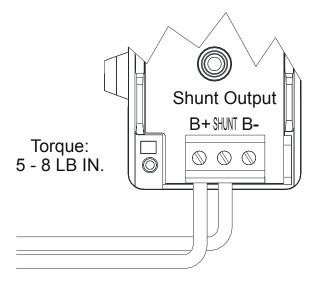
Figure 22: Power Module Shunt Wiring Diagram
