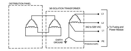
*Figure 20:* Three Phase Delta Distribution to a Three Phase Delta/Delta Isolation Transformer
