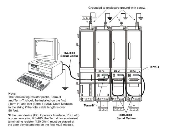
Figure 56: MDS Multi-Drop Wiring Diagram, RS-232 to RS-485 communications
