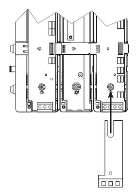
Figure 14: Installing the Optional Cable Strain Relief Bracket
