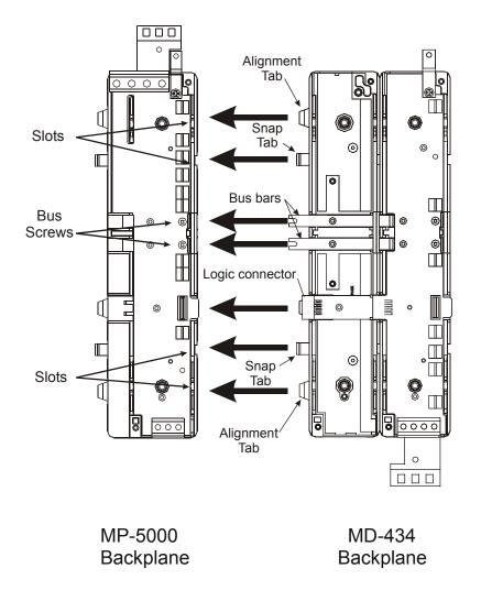
*Figure 12: Assembling the Drive Module Backplane to the Power Module Backplane.*
