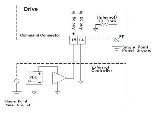
Figure 46: Analog Command, Single Ended Wiring Diagram
