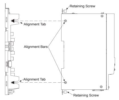
Figure 28: Drive Module Assembly Diagram
