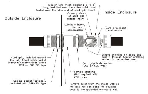
Figure 2: Through Wall Shield Grommet
