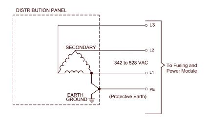
Figure 17: Earth Grounded Delta Distribution Transformer
