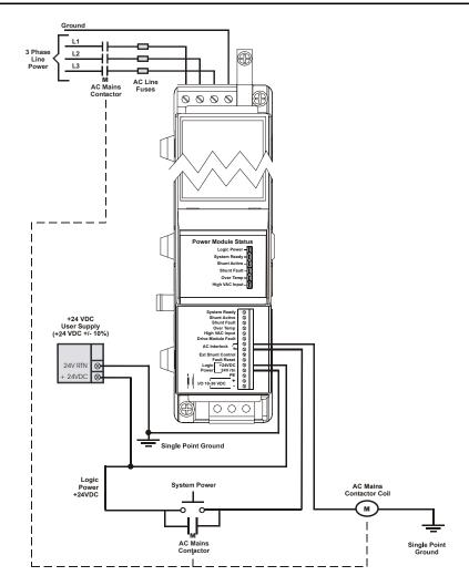
Figure 36: AC Interlock wiring with +24VDC Mains Contactor Coil
