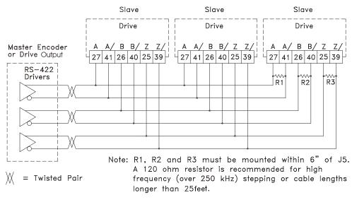
Figure 54: Master/Slave Encoder Connections
