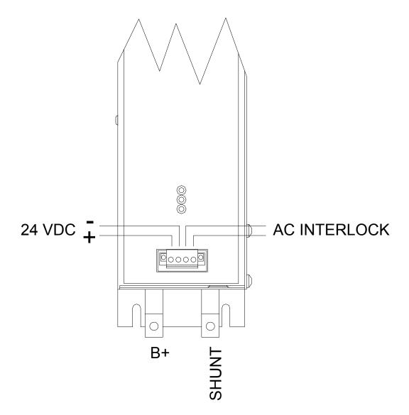
Figure 25: The MS-5XX-00 Connections
